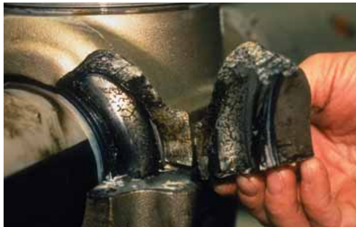
A cracked aluminum hub
