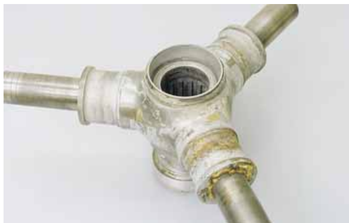
Corroded steel hub
