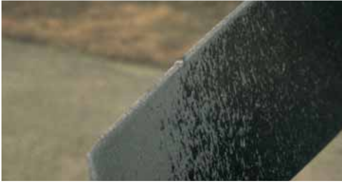
Blade erosion: Bare metal corrodes rapidly. Keeping blades properly painted is inexpensive routine maintenance.
