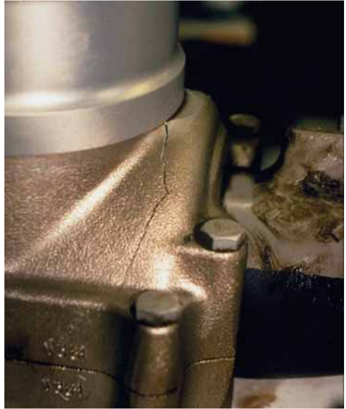
A cracked hub
