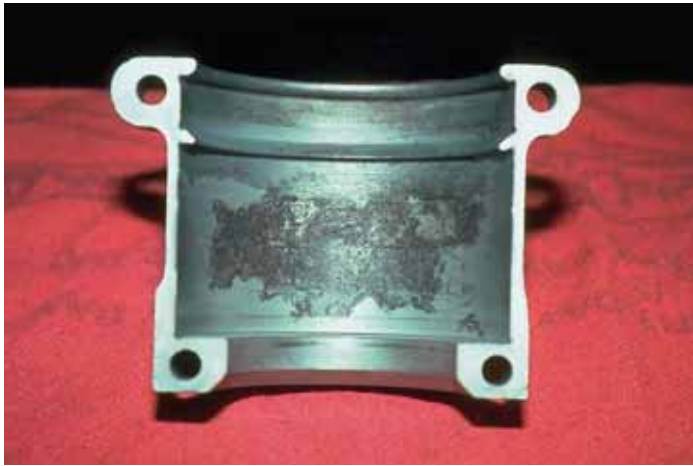
Corroded blade clamp
