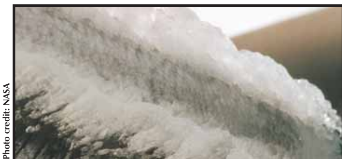
In-flight wing leading edge ice formation
