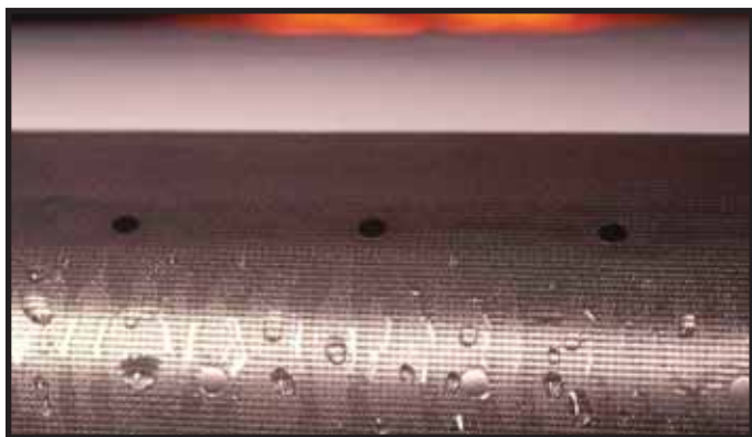
TKS patented alcohol deicer system
