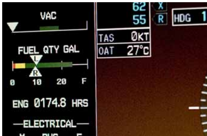
In glass-panel aircraft, fuel quantity may be shown on a multifunction display.
