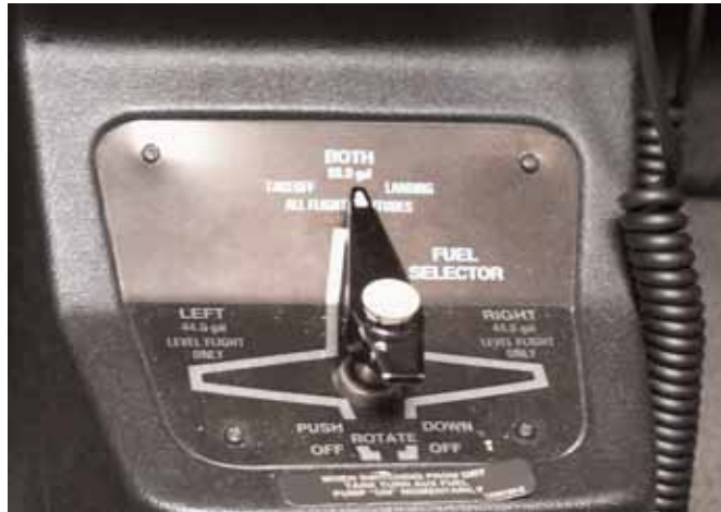
Fuel selectors on some aircraft can be difficult to see and manipulate, particularly in a dark cockpit.
