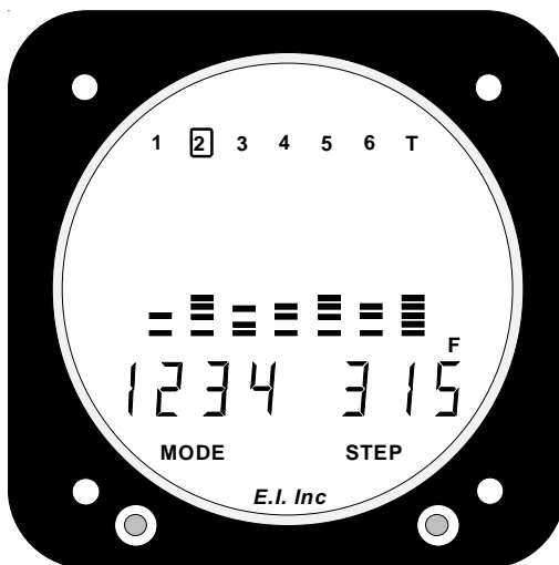
Fig. 17: Shows Normal mode with the engine operating at full rich.
