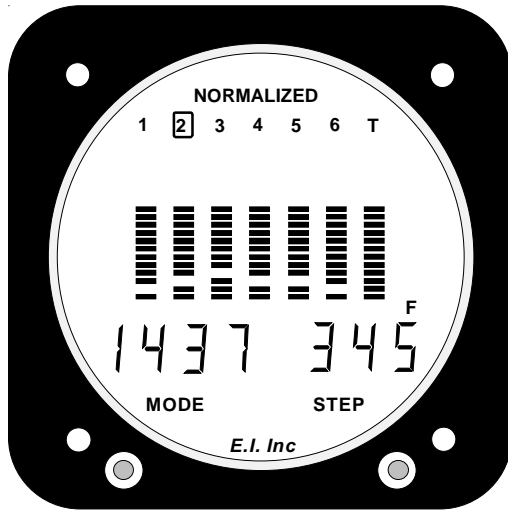
Fig. 15: Shows Normalized Mode with the engine operating normally.
