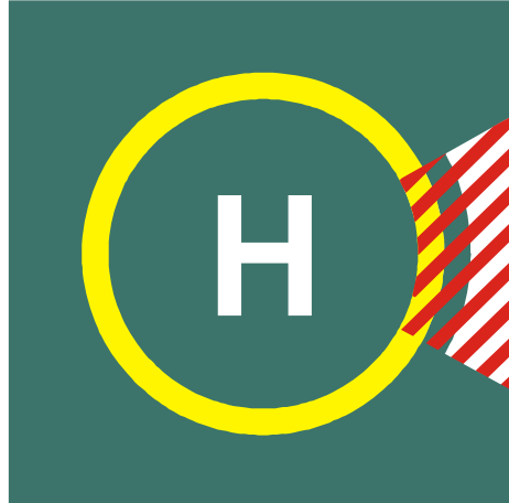
Figure 5-7. Helideck prohibited landing sector marking
