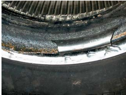
High Brake Heat Figure 312
