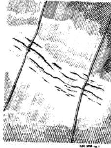
Tube Creasing Figure 315
