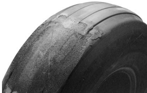
Wet Braking Flats Figure 305
